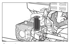
**Step 8** Adjust pressure control to desired setting.
